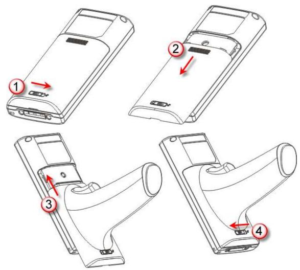
Figure 3: Installing the Pistol Grip
