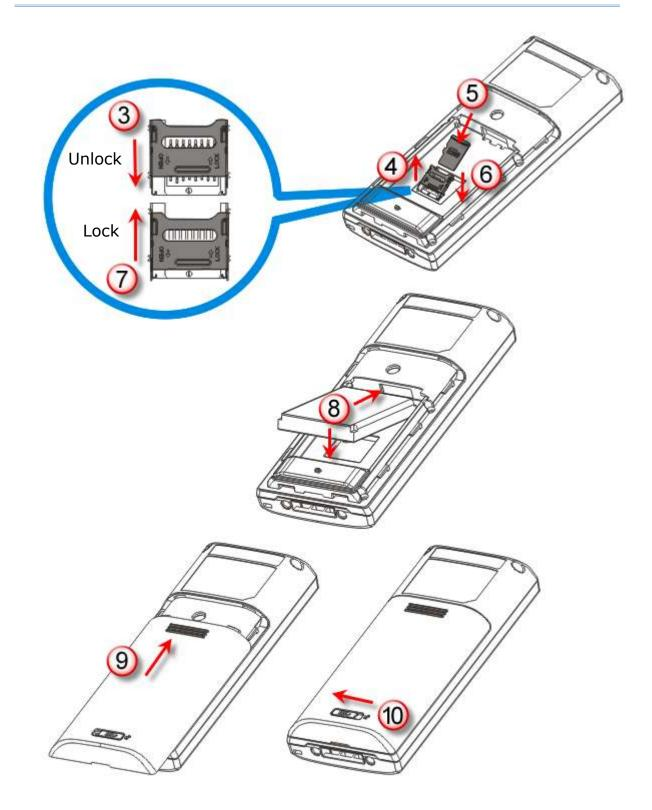
Figure 2: Installing the Main Battery & Memory Card
