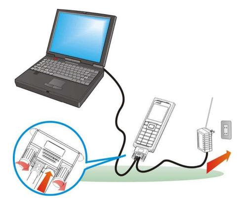
Figure 6: Using USB/RS-232 cable
